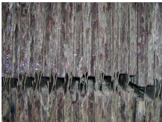
Fig. 6 – Biological film in the biodisk blades
