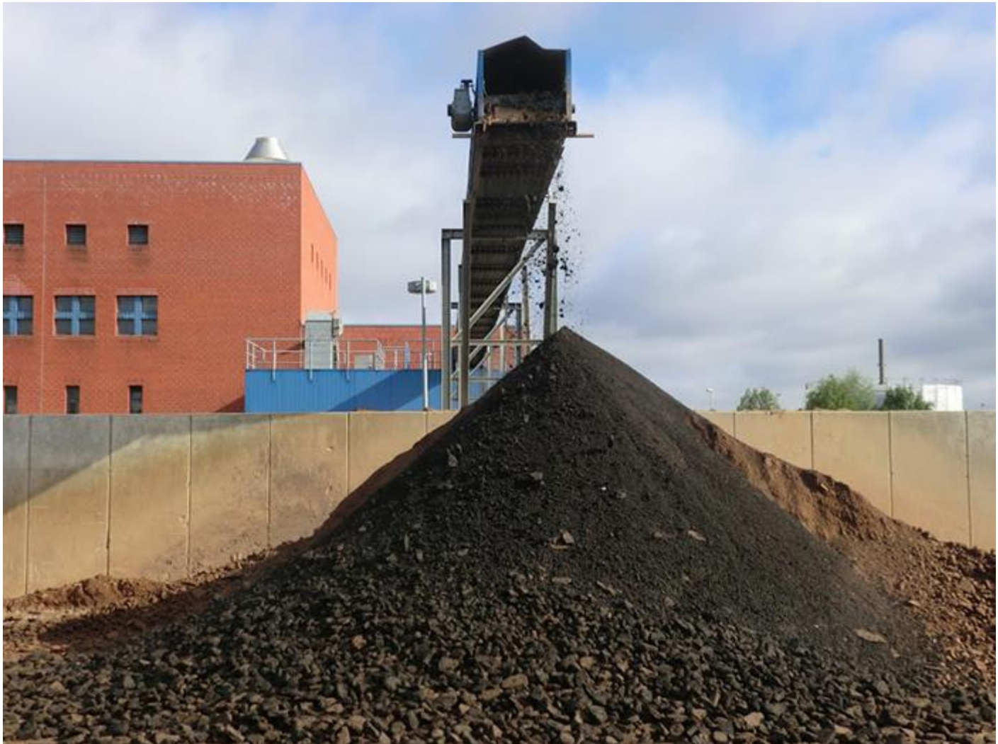
Sewage sludge, conditioned with milk of lime and then dewatered. Photos: Entsorgungsbetriebe Lübeck.
