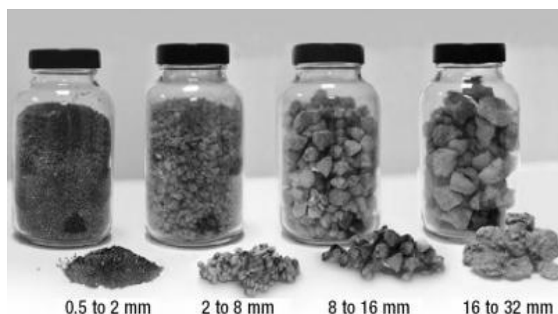
Figure 8: Bottom ash removed from the bottom of an incinerator (different particle sizes)
