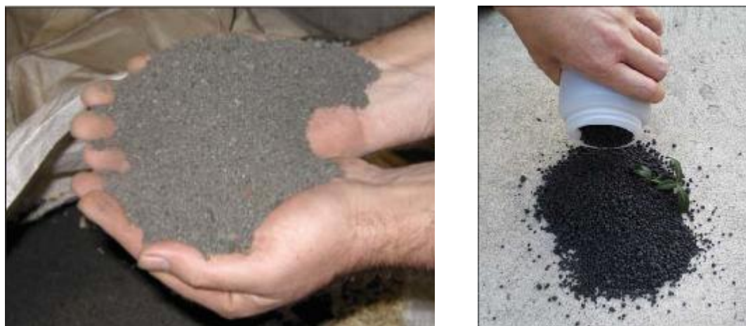
Figure 10: Pellets produced from sludge
