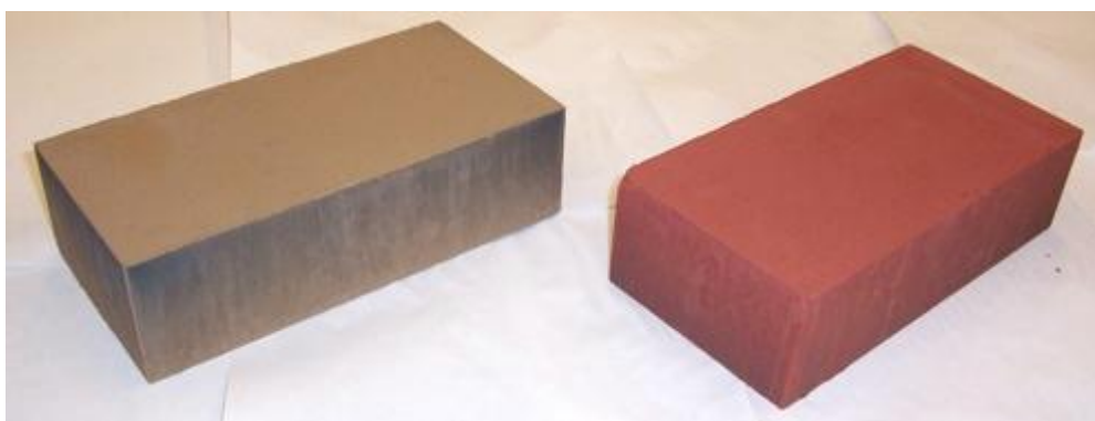
Figure 11: Bricks produced from sludge
