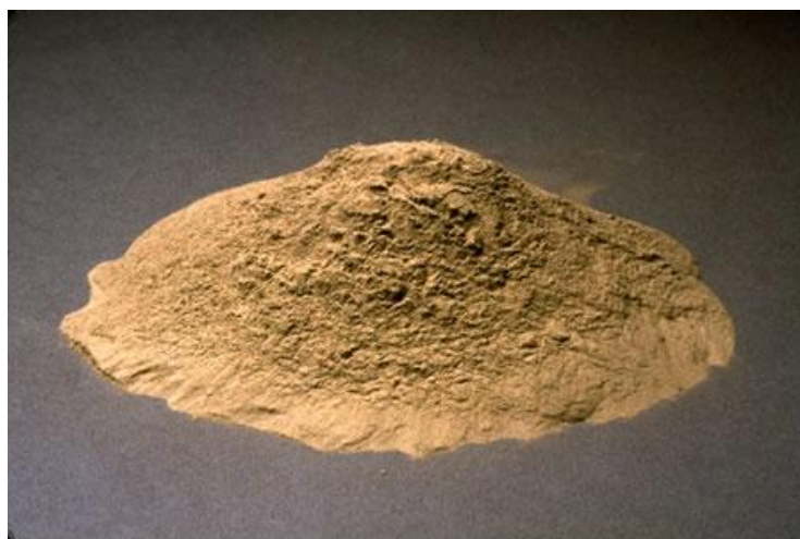
Figure 7: Fly ash recovered during sludge combustion
