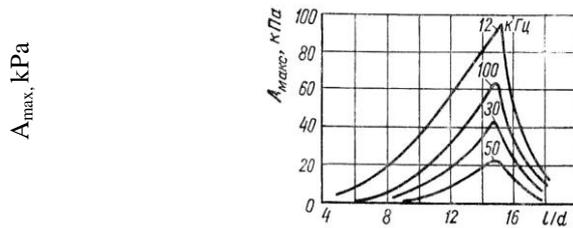
Fig. 22. Dependency of the maximum amplitude of accoustiv wave pressure on the  $l / d$  ratio for nickel ferromagnetic elements  $d = 1$  mm
