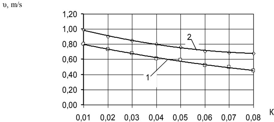
Fig. 20. Dependency of critical flow velocity on chamber filling coefficient
