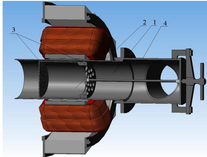
Fig. 7. The chamber of AVS for liquid phase processes:
