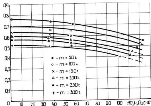
Fig. 17. Dependence of critical flow velocity on kinetic product viscosity coefficient ( $D_{\text{external}} = 76 \text{ mm}$ ;  $H = 11,8 \cdot 10^4 \text{ A/m}$ ; ferromagnetic elements: steel 08G2S,  $d = 2 \text{ mm}$ ,  $l/d = 10$ )
