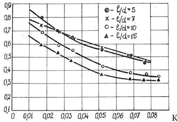
Fig. 15. Dependency of the critical flow velocity on the coefficient of chamber filling with ferromagnetic elements
