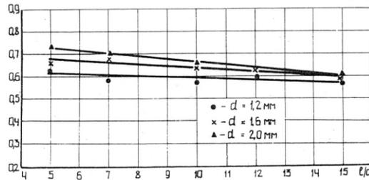
Fig. 16. Dependency of critical flow velocity on  $l/d$  ratio for various diameters of ferromagnetic elements ( $D_{\text{external}} = 76 \text{ mm}$ ;  $H = 11,8 \cdot 10^4 \text{ A/m}$ ); ferromagnetic elements: steel 08G2S,  $m = 150 \text{ g}$ )
