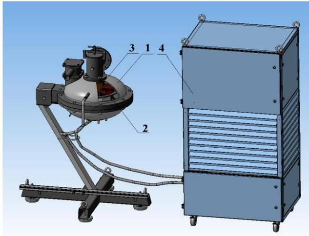
Fig. 2 AVS -150. Internal inductor diameter 150 mm, operating chamber diameter 136 mm.
