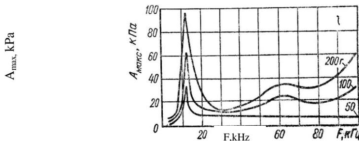
Fig. 24. Dependency of the maximum acoustic wave amplitude on the frequency of oscillations for ferromagnetic elements made of nickel wire with diameter  $d = 1$  mm and length of  $l = 15$  mm
