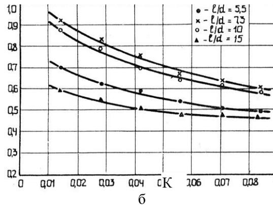
Fig.14. Dependency of critical flow velocity on chamber filling coefficient ( $D_{\text{ch}} = 76 \text{ mm}$ ;  $H = 11,8 \cdot 10^4 \text{ A/m}$ ), ferromagnetic elements:
