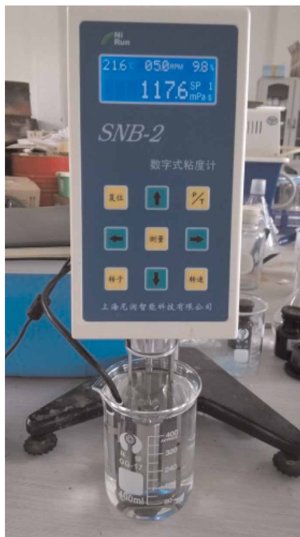
Figure 1 | The rheometer (SNB-2, Nirun, Shanghai, China) with geometrical dimensions of 370 × 325 × 280 mm.
